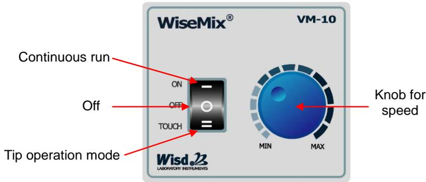
Continuous run: Set the switch “ON” for continuous mixing.
